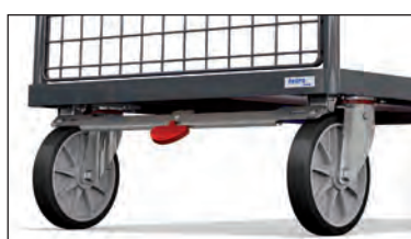
TOTALSTOP - the fetra central brake system With only one foot the rotation of wheels and the swivelling movement of both swivel castors can be securely locked. The brake pedal is always visible to the operator.
